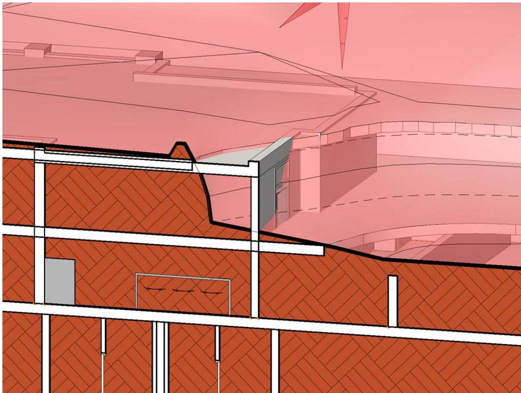
Cross section of proposed building showing effect of the irregular fall of the land with height intrusions (Rothelowman) in the area generally highlighted in the extract of the survey below.
